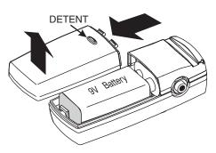
Figure 5: Battery Installation
